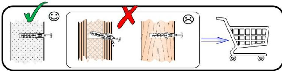
**-EN-** Before suspending or fixing furniture to the wall (in order to prevent falling over), check the type and strength of the wall. Select wall plugs and screws appropriate for the given type of the wall. In the case of doubts, contact a specialist. The installation must be performed by a competent person. **WARNING!!! If the rawplugs with screws are attached to the product, then they are intended only for walls made of solid and homogeneous materials.**
